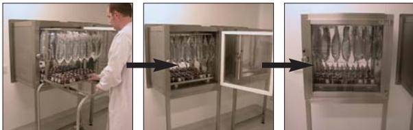
4. The trolley is wheeled to the relevant chamber where the rack can be simply pushed directly into the chamber and the door closed.
