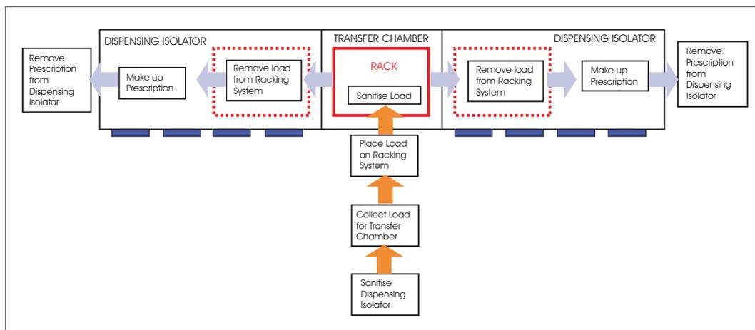
Figure 2: Rapid Gassing Chamber Process Flow Diagram.
