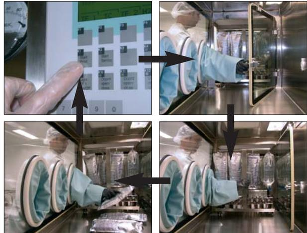
7. Once unloaded, the racks are passed back into the chamber for re-use and the door from the isolator to the chamber is closed and pneumatically sealed.
