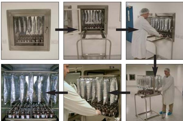
5. Each chamber has its own control panel mounted on the chamber front and on the push of a button, the door is pneumatically sealed and the cycle is initiated.
